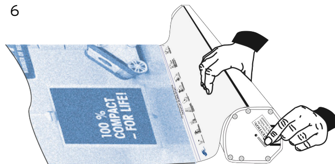
Hold the graphic panel and release the locking pin.
